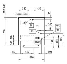
D = Drain ΕI Electrical connection
