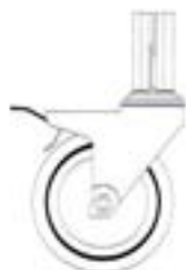
detail of swivel caster pintle mounted
