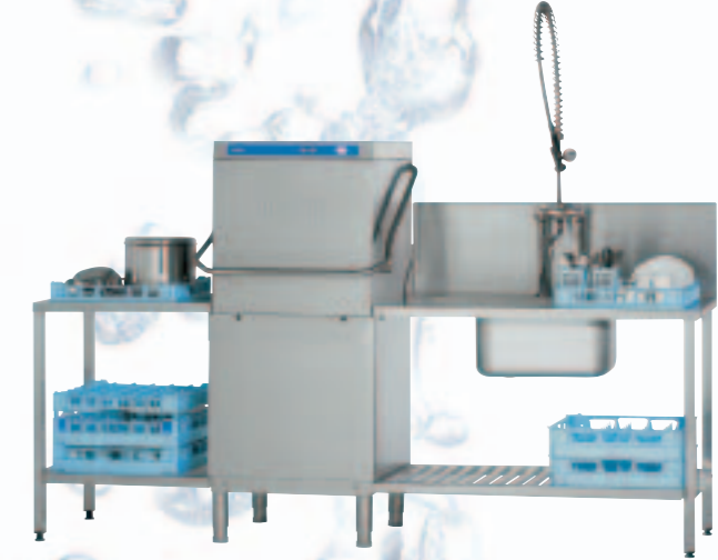
Model AUXX 1300 / AUXX 1300R Capacity – 70 cycles/hr Programmes – 52/90/240 sec. Rack dims. – 500 x 500mm Door opening height – 440mm
