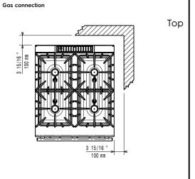
**Electric** Oven Heat Input: 8.5 kW Gas Gas Power: 48.5 kW 165336.5 Btu/hr Standard gas delivery: Natural Gas G20 (20mbar) Gas Type Option: LPG; Natural Gas Gas Inlet: 1/2"
